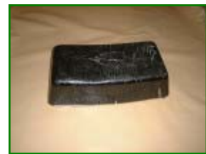
Modified-asphalt plate for bridge-floor waterproofing
